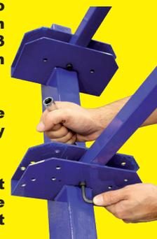
**3** Open the 2 side feet and insert the removable pin in the base frame hole following the selected configuration.
